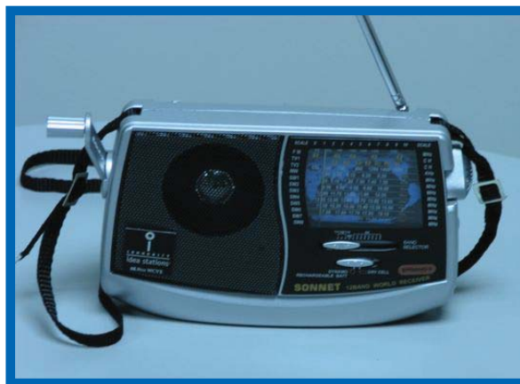
Crank-powered radio which can be used during power outages. This will be an important part of improved emergency communications.
